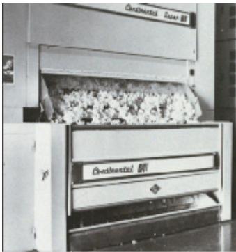
Revolving Circular Saws Pull Lint from Seed in the Ginning Process
